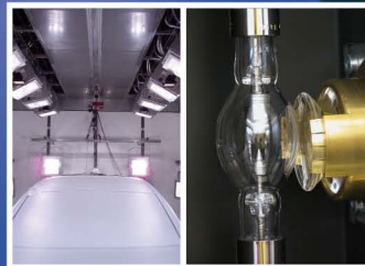
(left) Solar and weathering simulation for car bodywork (right) XBO lamp with lenses for solar simulation
